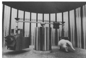
Fig. 1. Apparatus for spacing motion and convergent visual feedback for an actively moving and a passively moved animal. (Photograph by T. Palanichamy.)
